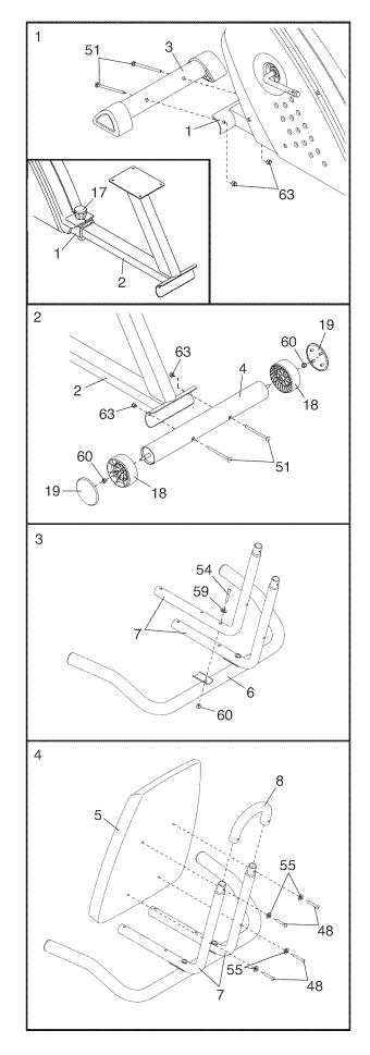
Have another person hold the Seat Frames (7) under the Rear Frame (2) as shown. Attach the Seat Frames and the Seat (12) to the Rear Frame with four M6 x 42mm Button Screws (49) and four M6 Washers (55).
